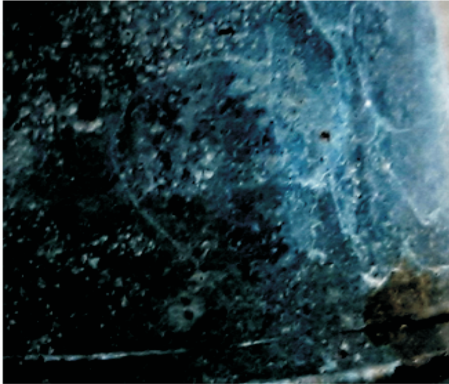
Figure 3- Material of pipe after exposure to water sample no 17
